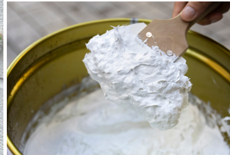
Left: SUZUKI Masaomi, CEO of Aster Co., Ltd., applies Aster Power Coating to a wall using a roller. ASTER Below: Aster Power Coating contains both glass fiber and acrylic silicone resin.
