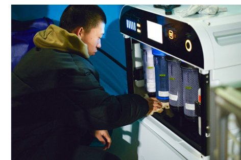
Top left: A middle school student carrying out maintenance on the inside of a WOTA BOX at an evacuation center in Noto.
