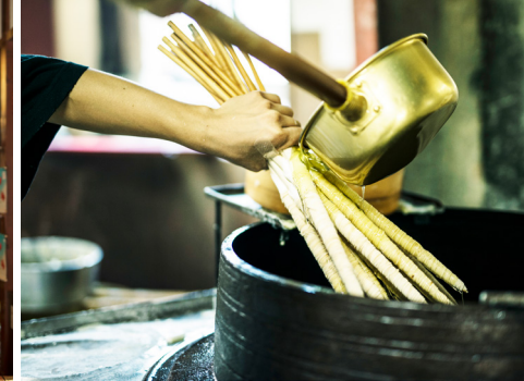
Left: TAKAZAWA Hisashi runs Takazawa Candle. This photo from before the earthquake shows the historical store's former interior. Right: The shinjime process for applying melted wax to the wick of a Japanese candle. The wick is covered with a thin layer of wax prior to being processed into a candle to prevent it from falling apart.
