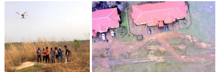
Left: Drone flight tests in Sierra Leone. Since multicopter drones have an advantage over fixed-wing drones in terms of imaging accuracy, both may be used depending on the situation.
