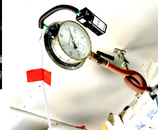
The IntegrAI system is ready to go after simply attaching a camera to an instrument.
