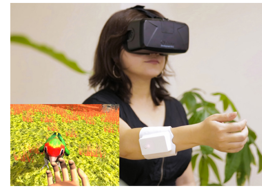
Conveying proprioceptive sensations to the body by sending electrical stimuli through a white band worn on the arm, UnlimitedHand can realistically reproduce the weight and presence of a small bird (bottom left) held in the hand. H2L
