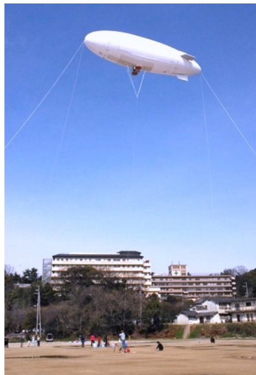
The photo shows a microwave wireless power-transfer experiment from an airship to the ground, conducted by Kyoto University in 2009. Due to its ability to send and receive power over longer distances than other contactless power-transfer methods, the technology to wirelessly transmit power with microwaves shows promise for use in a variety of applications on the ground, such as supplying power to disaster areas where infrastructure has been disrupted.
