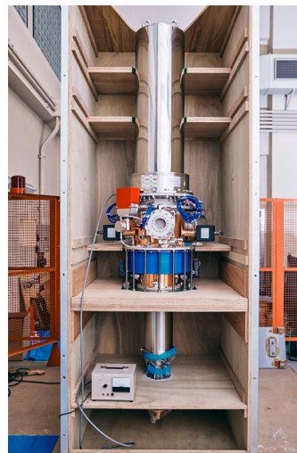
A gyrotron, a special machine that heats the plasma fuel with microwaves to 100 million degrees Celsius or higher. It operates in a similar way to an extremely powerful microwave oven.
